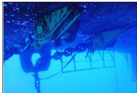
Figure 5: Towing gear (capsized barge)
