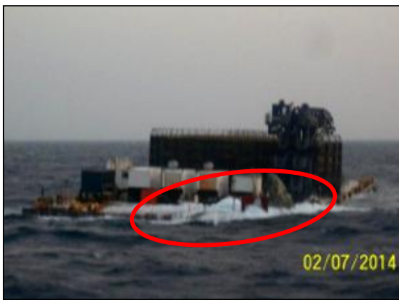
Figure 3: Green seas shipped on the open deck from port side
