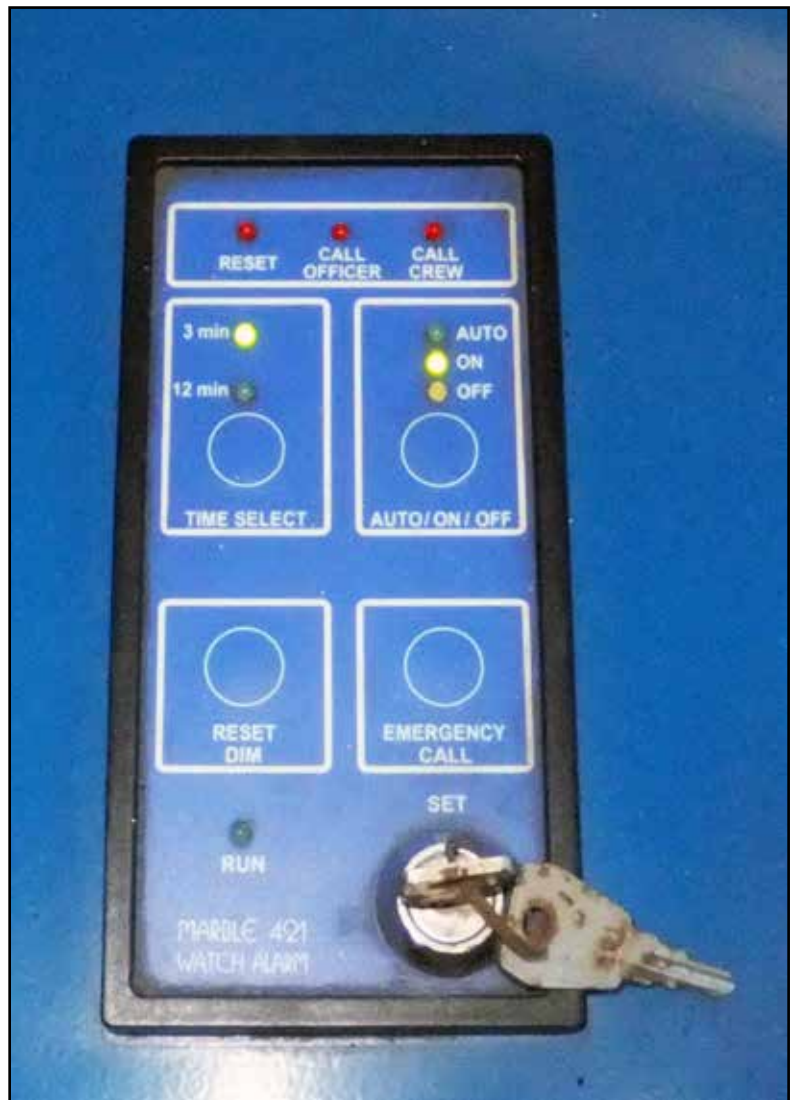
Figure 2: Bridge navigation watch alarm system's control
